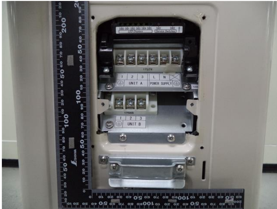
161. RAS-2M14U2AVG-E, Terminal block for interconnecting cable and cord anchorage
