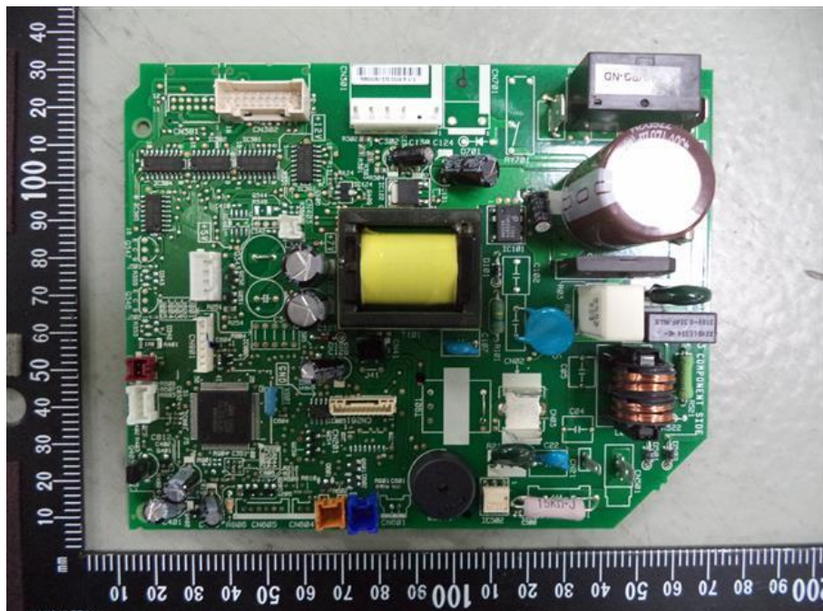
44. RAS-M10PKVPG-E, Main PCB component side
