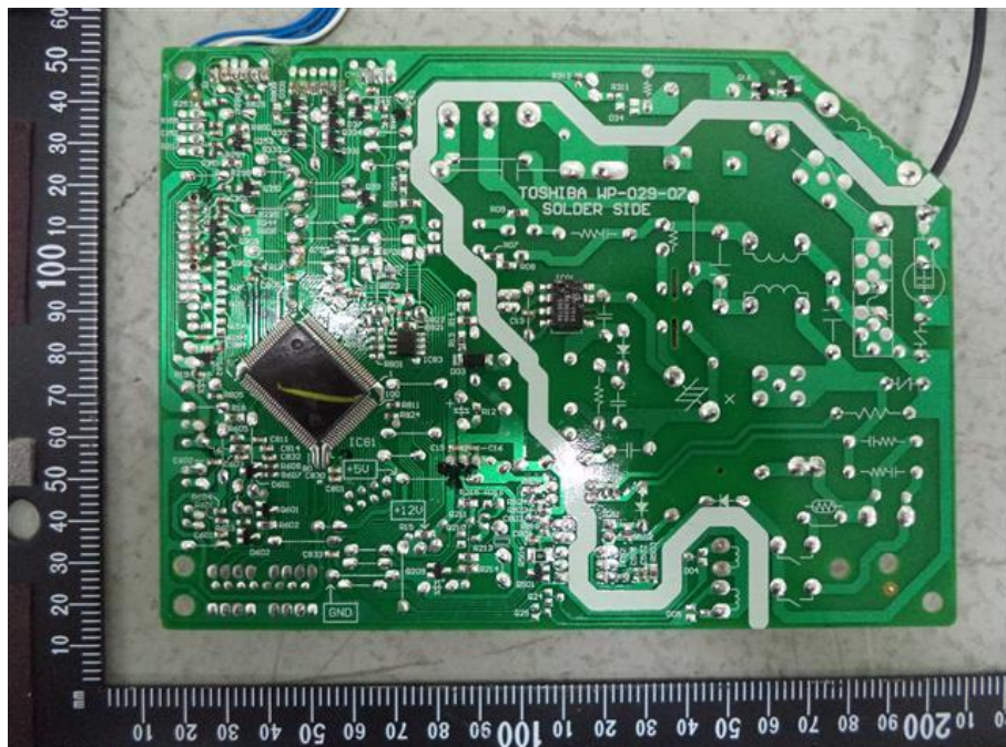
74. RAS-B07BKVG-E, Main PCB soldering side
