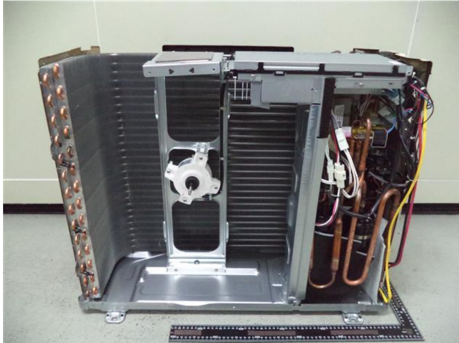
135. RAS-2M10U2AVG-E, Internal view removed fan blade
