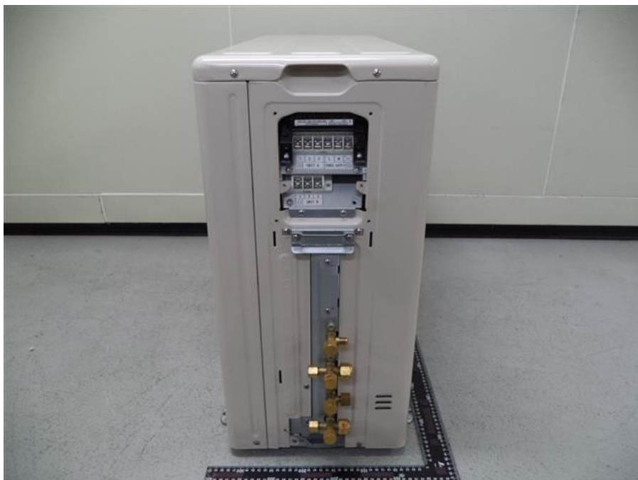
130. RAS-2M10U2AVG-E, Terminal block for supply main, interconnecting cable and cord anchorage
