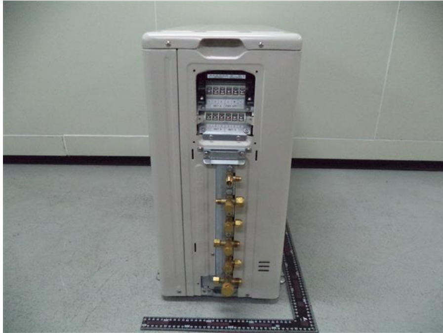
181. RAS-3M18U2AVG-E, Terminal block for interconnecting cable and cord anchorage
