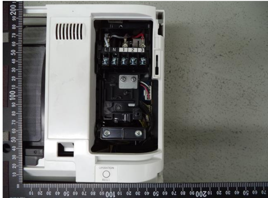
61. RAS-B07BKVG-E, Terminal supply, interconnecting terminal and cord anchorage
